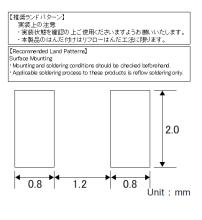
The data is reference only. Electrical characteristics vary depending on environment or measurement condition. TAIYO YUDEN reserves the right to make change to the data at any time without notice. Before making final selection, please check product specification. 2019.01.04
